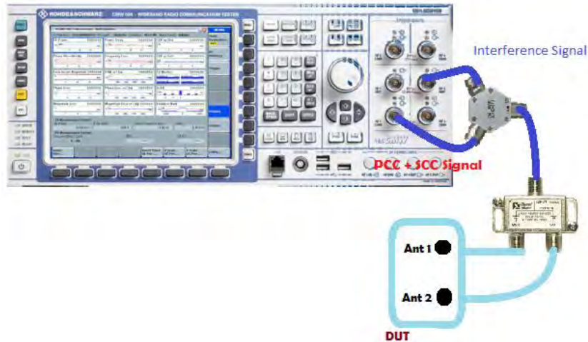
Fig. 11: Setup for testing with an internal interference generator.
